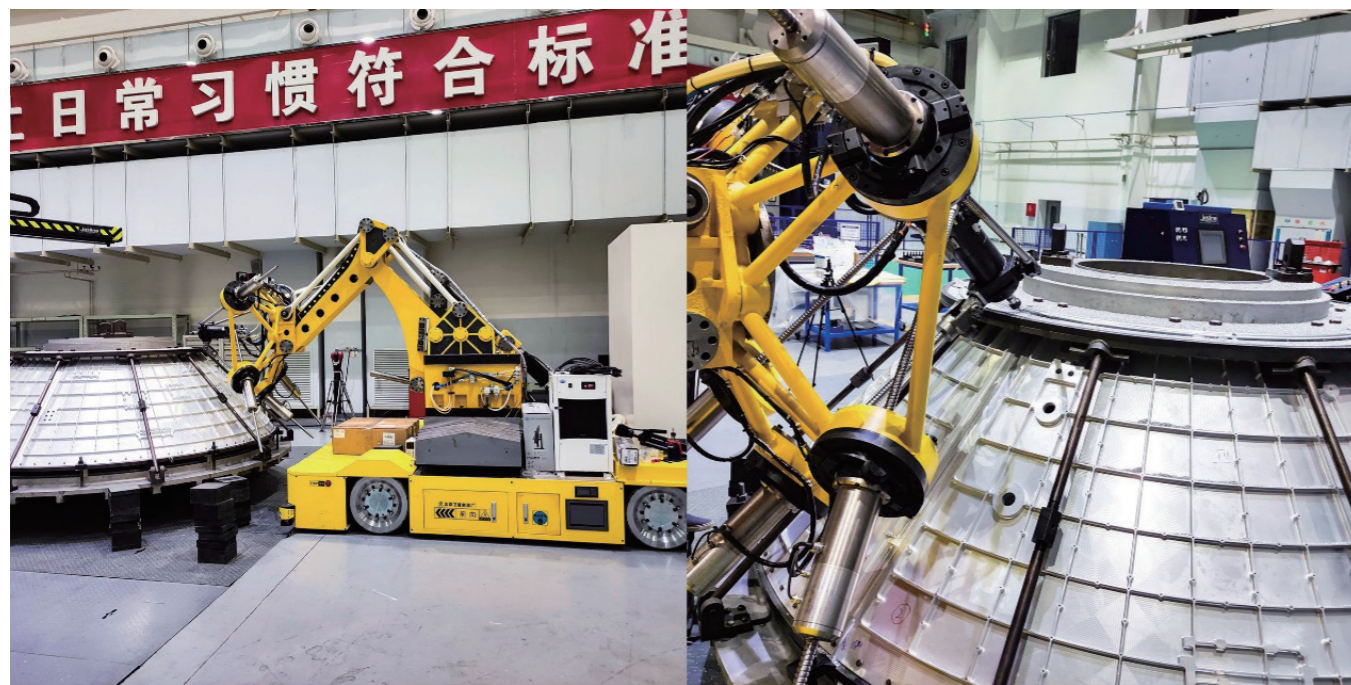
In-situ machining of Tianzhou-6' conical segment
